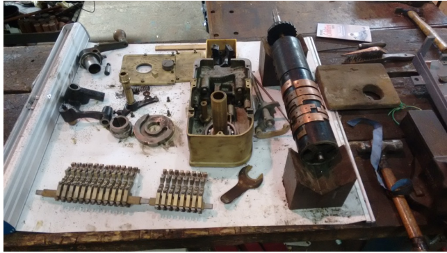
Coronation controller ready for refurbishment
